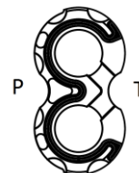
6°- Be sure that the plate seal is assembled on the pressure side (P side). Be aware that the seal tips should not be damaged when inserting the plate
